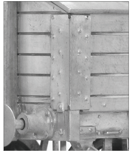
Note how the buffer beam folds around and how the corner plate is positioned relative to plank lines.
